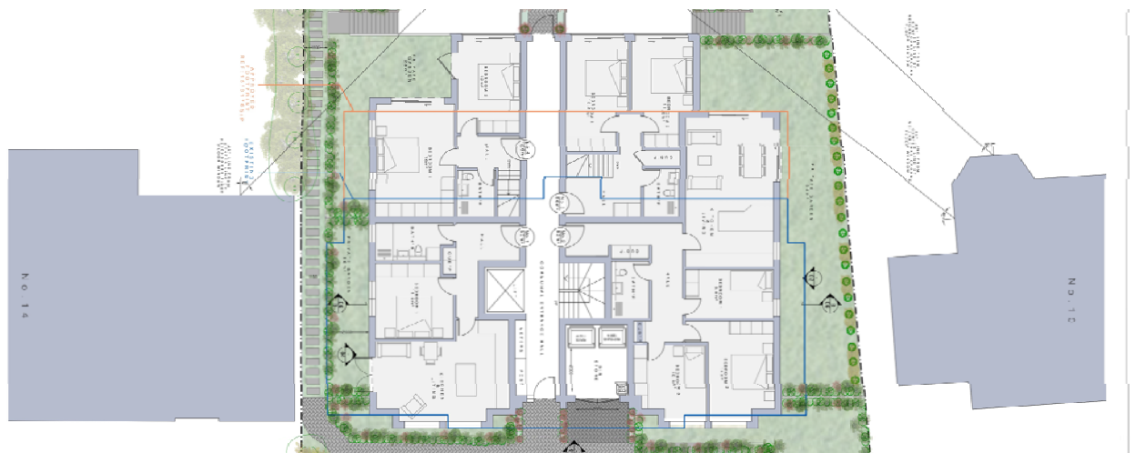
Figure 5: Proposed Ground Floor Plan with existing footprint indicated with blue line and orange line indicating the previous consents
